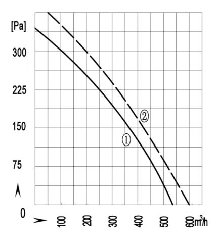
Curve 1: 50HZ Curve 2: 60HZ
